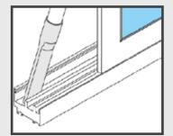
For GOS-S windows, in order to enable excellent drainage of the water, periodically clean or vacuum the area by the T-REX water evacuation plug.
