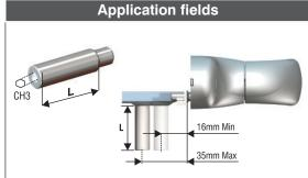
Note: New connection pins in Silver Plus GS The 3 mm hexagon impression facilitates screwing the pins on the slider.
