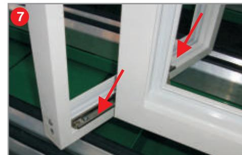
7 Final mounting of the arm to the frame after adjustment
