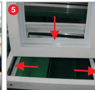
5 Fitting the sash and drilling the mounting holes in the frame
